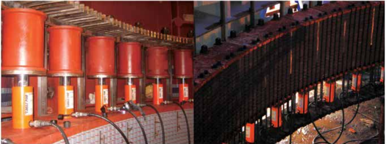
106 EAGLE PRO ES-306 single acting cylinders are used to press the laminates into the stator core hold down gear.
