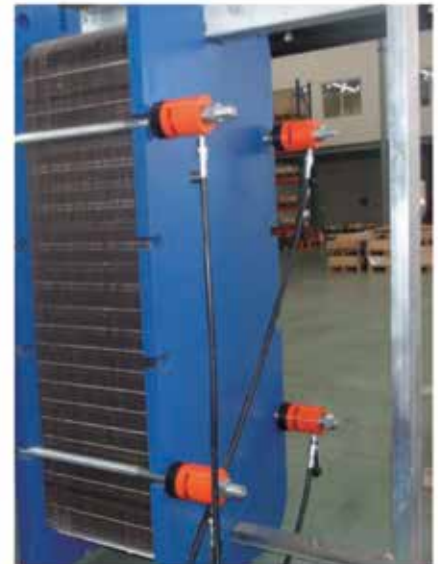
4 EAGLE PRO ESH-306 pulling threaded bar in a the largest heat exchanger in SONDEX's factory in Ningbo China.
